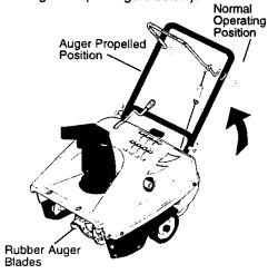
**CAUTION:** Read owner's manual before operating machine. Never direct discharge toward bystanders. Release the auger control bar and stop the engine before unclogging discharge chute or auger housing and before leaving the machine.
